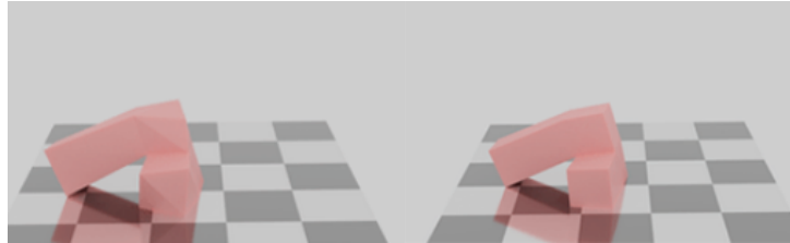
Figure 2: Left is the explicit time integration method, right is the implicit time integration method. The implicit time integration method is more stable than the explicit time integration method.
